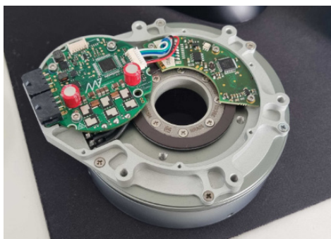
AksIM encoder integrated in the MA-hs actuator
