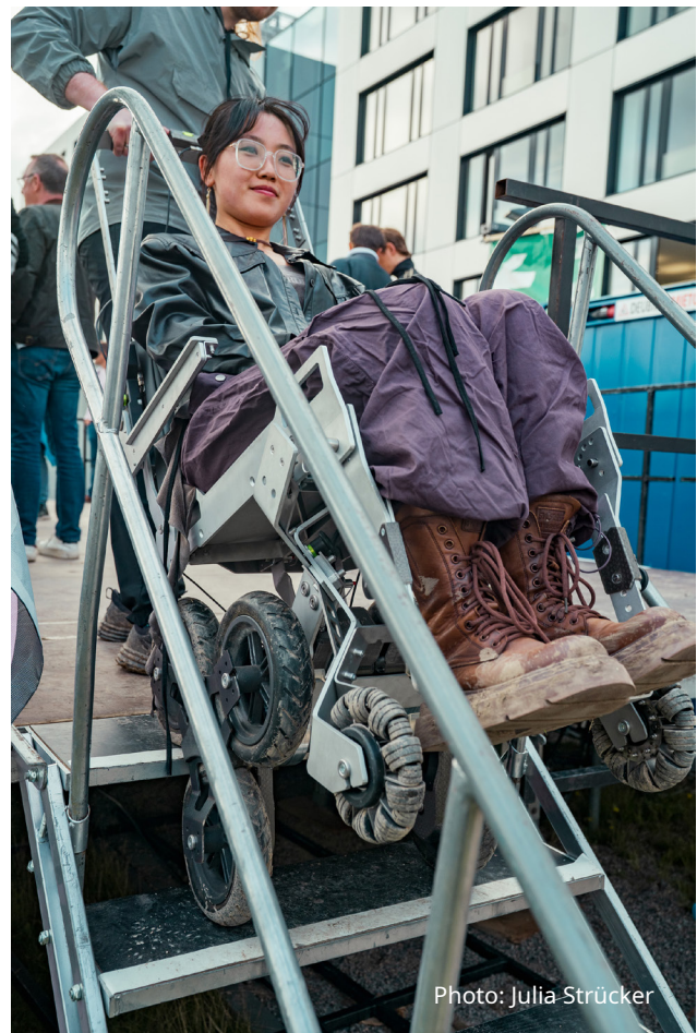
Electrically assisted stair-climbing transport aid
